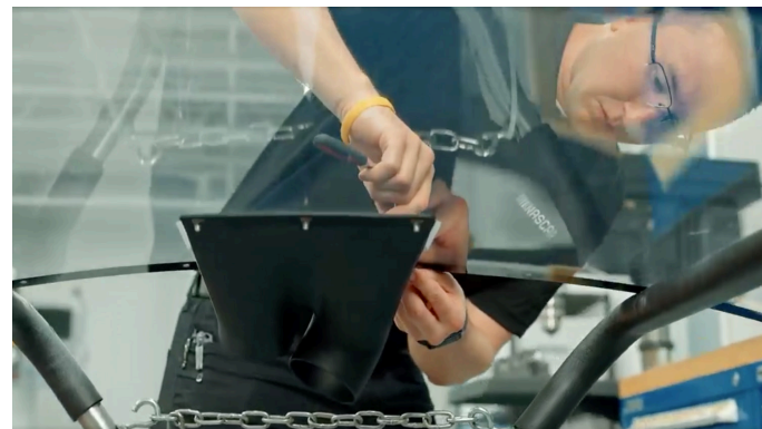
Tim Murphy, part designer, installs air flow duct onto Next Gen car windshield.
