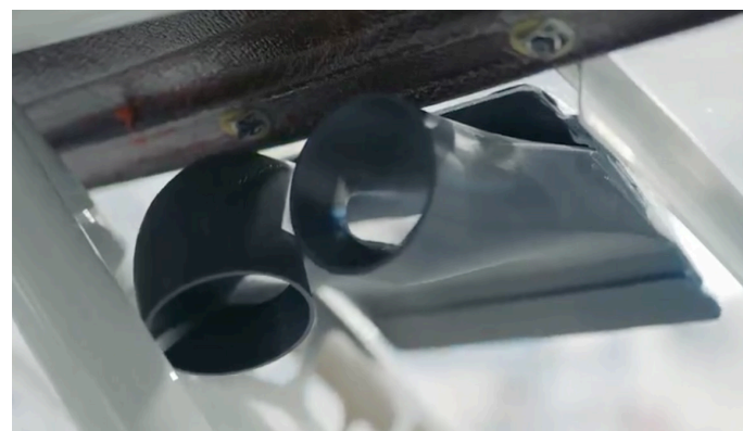
Tim Murphy, part designer, installs air flow duct onto Next Gen car windshield.
